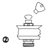
Adjust the required flow volume by turning the regulating spindle to the left (see diagram).
