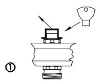
Remove the plastic cap and close the valve by turning to the right using a bleed key (close = smallest volume).
