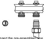
Insert the pre-assembled ppe into the screw connection.
