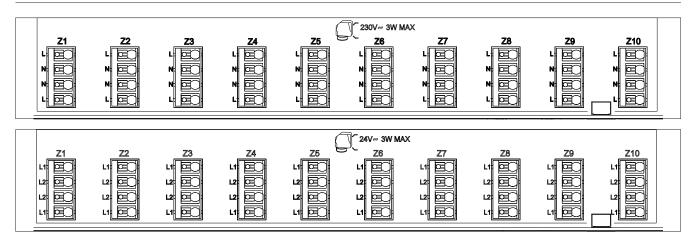
Connect one NC or NO actuator per connector.
