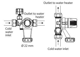
BI15 can be installed either vertical or horizontal position
