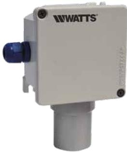
Gas detector sensor in metal housing (Group II protection mode, category 3G, Ex nA IIC T6) with operating status indicator LED for indicating gas alarms by means of a 4-20 mA analogue output or a trip threshold (pre-alarm, level 1 and 2 alarm, fault) that can be freely set with DIP switches.
