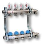
Stainless steel round-tube manifold for 2 up to 12 heating circuits for distribution, shutoff and balancing of the heating/cooling water flow of radiant panel heating/cooling systems in compliance with BS EN 1264-4. The flow rate for each heating circuit can be continuously adjusted via a regulating shut-off valve integrated in the return circuit. The inspection glasses integrated into the manifold's supply enable visual function checks.
