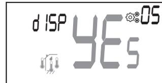
➤ “no”: thermostat displays set point temperature
