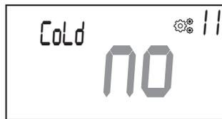
This parameter menu appears only if digital thermostat is associated with a Touch screen BT-CT03 or a 6Z or 10Z connecting box.
