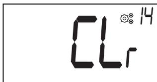
Press and hold
