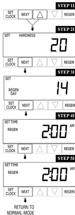
**STEP 4I** – Next Regeneration Time (hour): Set the hour of day for regeneration using the DOWN or UP arrow. AM/PM toggles after 12. The default time is 2:00 a.m. This display shows REGEN ON 0 GAL if ON 0 is selected in Step 9S or Step 7F. Press NEXT to go to step 5I. Press REGEN to return to previous step.
