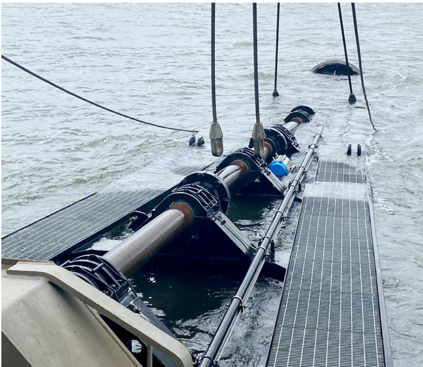
Safe working pneumatic actuators are managing every situation whenever the dredging boom is above or below water.
