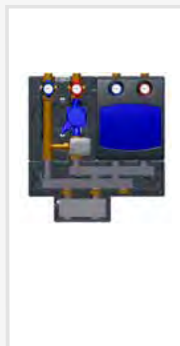
Connection with HW-Q60/80 and primary flow on left
