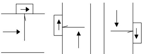
Before installing push the paddle slowly, allow it to return slowly, the switch should operate. Ensure the arrow on the housing points in the direction of the flow.
