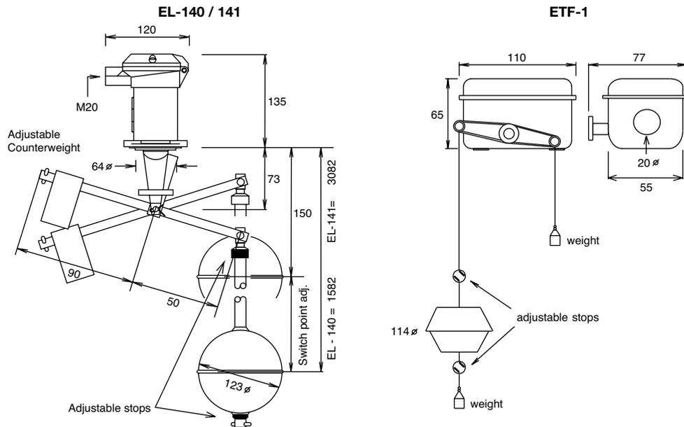
When float reaches upper adj stop C-NC close : When float reaches lower adj stop C-NO close
