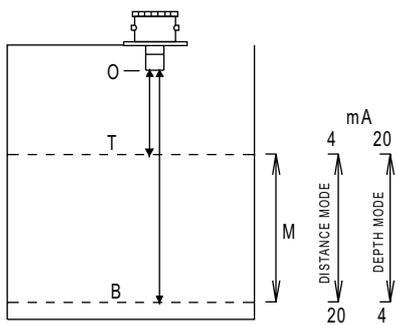
The unit can be set to read in either Distance or Depth mode.
