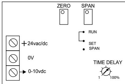
Link RUN for normal operation and 0vdc adjustment.
