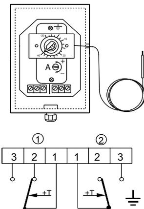
Diff between stages adjust via screw A
