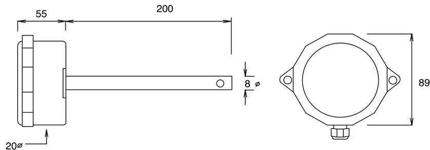
Ensure that the air flows directly through the holes in the side of the probe. The air can enter the holes from either side. Mount away from bends, elbows and turbulent areas. Avoid installing in areas where the temperature in the duct changes rapidly. DO NOT SUBJECT THE SENSING ELEMENT TO OILY, DIRTY, DUSTY OR MOIST MEDIA.
