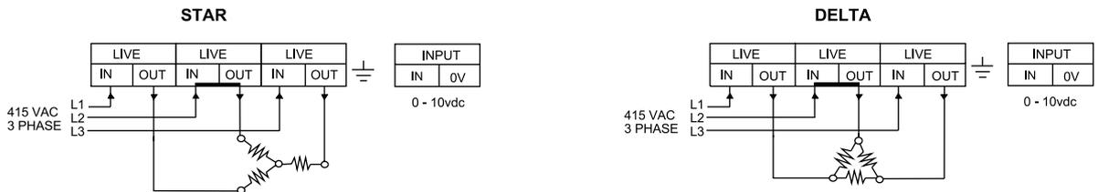
For Normal use the MAN/AUTO link should be on AUTO. In MANUAL the potentiometer is used to regulate the output.
