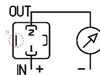
Min sensor / control signal cable size 7/0.2mm
