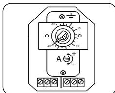
Diff between stages adjust via screw A
