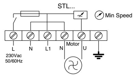
L1 : Live supply bypassing the Fuse & On/Off switch (which is on the side) or it can be used as a supply for 3 wire motors.
