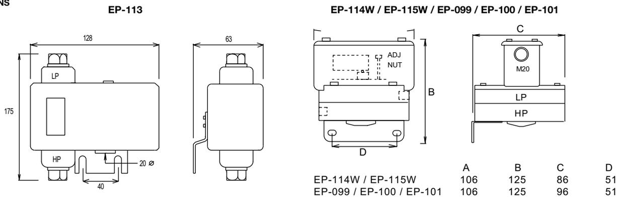
Mounting at any angle is possible. HP = High Pressure bottom port LP = Low Pressure top port
