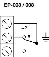
**EP.** On pressure rise to scale setting (range) 1-4 close .. On pressure fall (diff) contacts 1-2 close.
