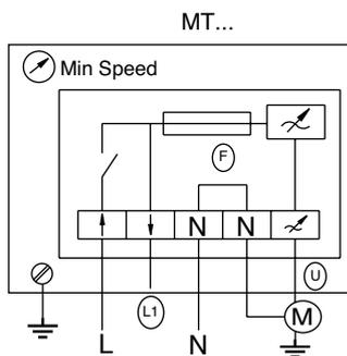
L - Live supply via On/Off switch: 230Vac
