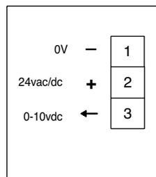
**INSTALLATION:** Terminals 0.5-2.5mm      Min sensor / control signal cable size 7/0.2mm      Max length 100m.
