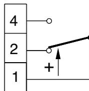
On detection of condensation contacts 1-2 open and 1-4 close.
