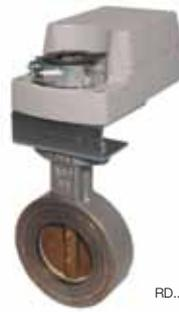
Materials: Cast Iron Body, Brass disc, Stainless Steel spindle, Graphite asbestos packing gland.
