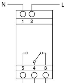
The live connector must be protected with a MCB or fuse of max 16A.
