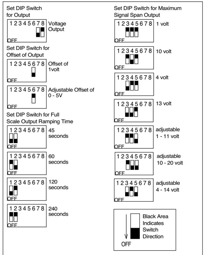
B.M.S RESISTANCE INPUT MODULE 135/1000Ω IN 0-10VDC OUT
