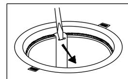
Rotation angle is adjusted by repositioning the adapter in 5 steps. The adaptor is released by pressing the locking clip on the underside of the actuator.
