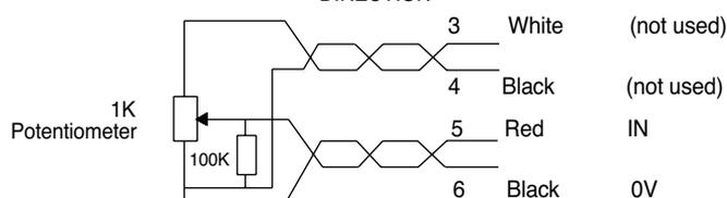
The 3m cable can be extended using screened 7/0.2mm wire equivalent to Belden 9503. The screen is not connected in the sensor and should be earthed at the controller end. Keep away from power cables/units which may cause interference.
