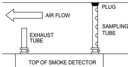
Fit the sampling tube across the entire width of the duct. The tube can be cut to the required length. Minimum duct width 200mm. FIT THE PLUG PROVIDED TO THE END OF THE SAMPLING TUBE. The holes in the sampling tube should face towards the air flow. ΔP between input & exhaust tubes should be between 0.024 to 3.0 mbar. An exhaust tube is provided – this must not be blocked. The tubes & air flow direction can be reversed.
