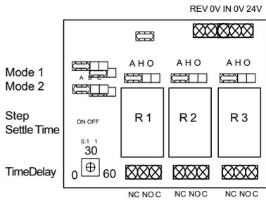
Time Delay : Allows a time period before each stage switches on or off. Set to 0 if not required.
