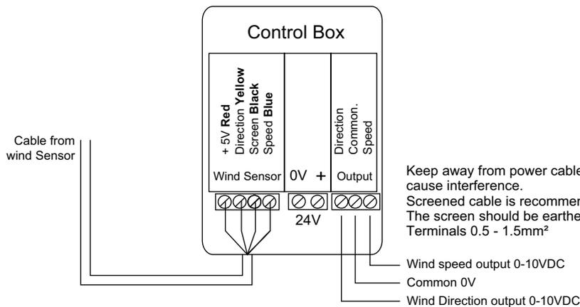
Supplied with the control box which converts the sensor signal to a standard 0-10 volt output signal.
