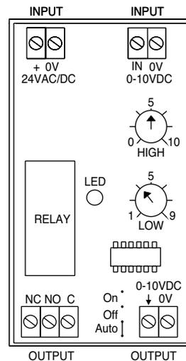
When the 0-10vdc input signal increases to the High setting contacts C-NO close.
