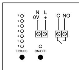
Select the run time required by repeatedly pressing the HOURS button and the corresponding LEDs will turn on. These LEDs will also turn off in sequence during the countdown period. Push the ON/OFF button, contacts C-NO close and the ON/OFF LED turns on to indicate run time has been extended.
