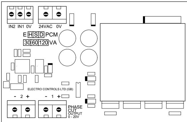
For the 24VAC POWER SUPPLY select transformer VA rating according to actuator rating.
