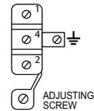
**Adjustment :** Units are pre-set to the approx. minimum setting. Adjusting below this value may result in the switch failing to return To increase switch point, slowly turn adjusting screw **CLOCKWISE**
