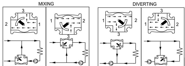
The motor can operate between ports 3-2 or 3-1
