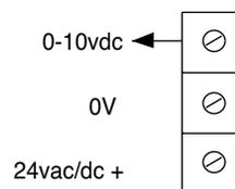
**INSTALLATION:** Terminals 0.5 -2.5mm      Min sensor / control signal cable size 7/0.2mm      Max length 100m
