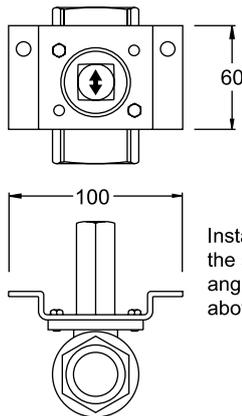
Install the valve with the spindle at any angle vertical to 30° above horizontal.
