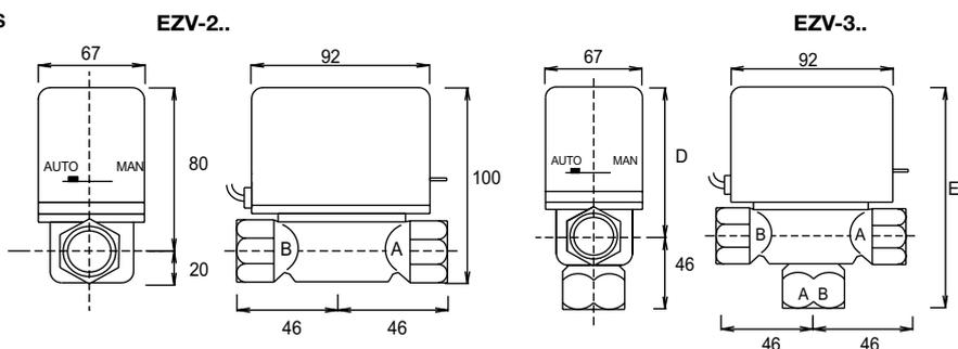
Install the valve with the motor at any angle vertical to 30° above the horizontal plane.
