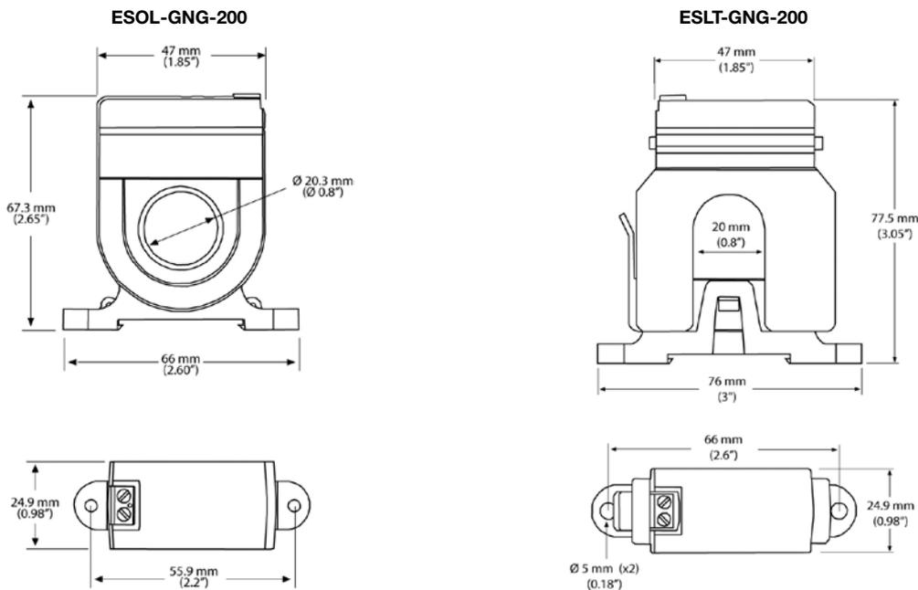
**INSTALLATION:** Ensure core is clean at time of installation as dirt/foreign particles may prevent correct operation. The split core device can be opened by using a large blade screwdriver positioned in the centre of the latch. When closing the split core ensure that the two halves are properly aligned. Pass the live conductor/wire through the core.
