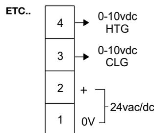
**INSTALLATION:** Terminals 0.5-2.5mm<sup>2</sup> Sensor cable size 7/0.2mm Keep away from power cables/units which may cause interference. Max length 100m. Screened cable is recommended. The screen should be earthed at the controller end only .
