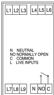
When a signal is received on any input - volt free contacts C-NO close
