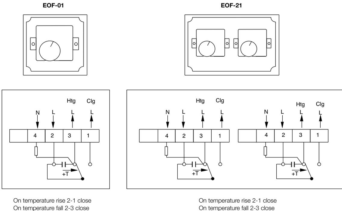
**INSTALLATION:** Outside Thermostats & Sensors which are used for frost protection should be mounted on the North side of the building. If this is not possible, shield the sensor from direct sunlight.
