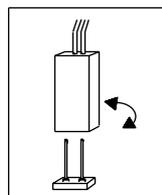
The direction of rotation is changed by reversing the polarity of the motor plug.
