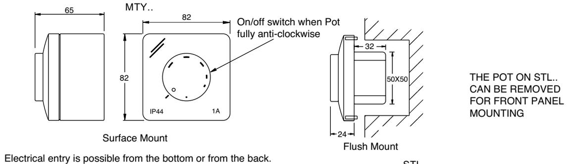
Electrical entry is possible from the bottom or from the back.
