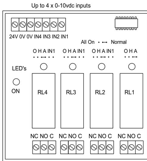
Each 0-10vdc input and relay output is independent. Outputs 1,2,3 or 4 can be linked to just one input IN1.
