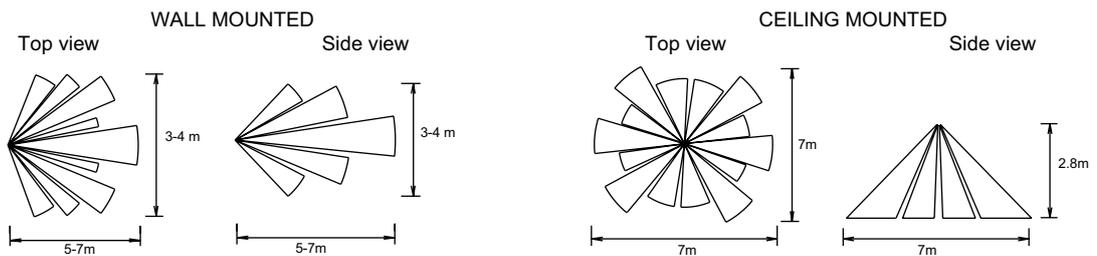
DO NOT MOUNT IN DIRECT SUNLIGHT OR NEAR HEAT SOURCES. In larger areas wire more switches in parallel to power the load.
