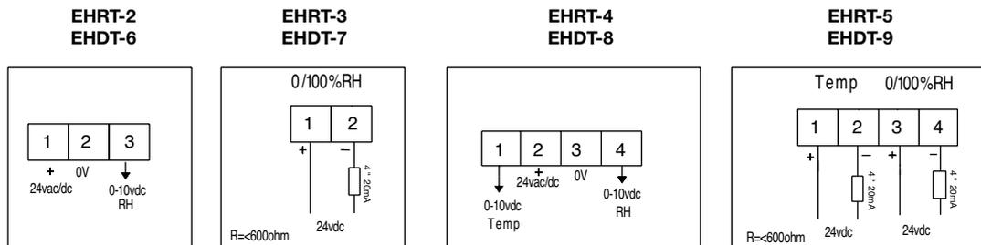
**INSTALLATION:** Min sensor / control signal cable size 7/0.2mm Max length 100m. Keep away from power cables/units which may cause interference.
