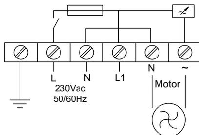
L - Live supply via On/ Off switch & fuse
