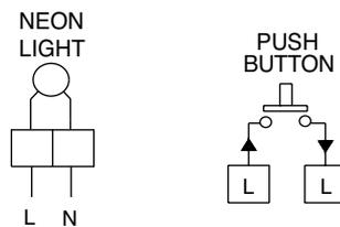
When the momentary action push button is pressed a circuit is made.
