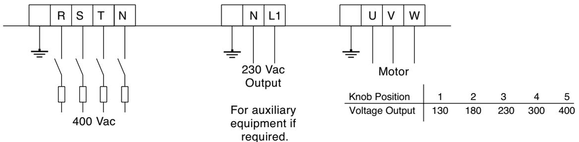
All cables & external fuses must be fitted according to local regulations, safety and motor manufacturers requirements.
