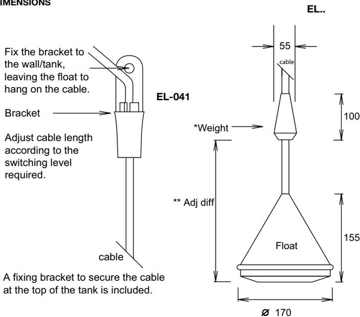
\*EL-AL & EL-AH do not use a weight. The switching point can be set by adjusting the length of cable in the tank.
