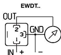
Min sensor / control signal cable size 7/0.2mm
