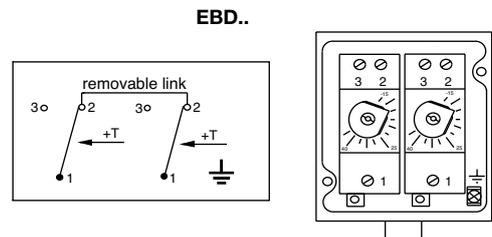
OPEN HIGH Contact 1-2 opens on temp rise. Temp must fall to allow resetting
