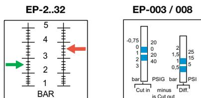
**EP-2..32** : Set the RED arrow FIRST to the High switch point, then set the GREEN arrow to the Low switch point. The differential is RED minus GREEN setting.
