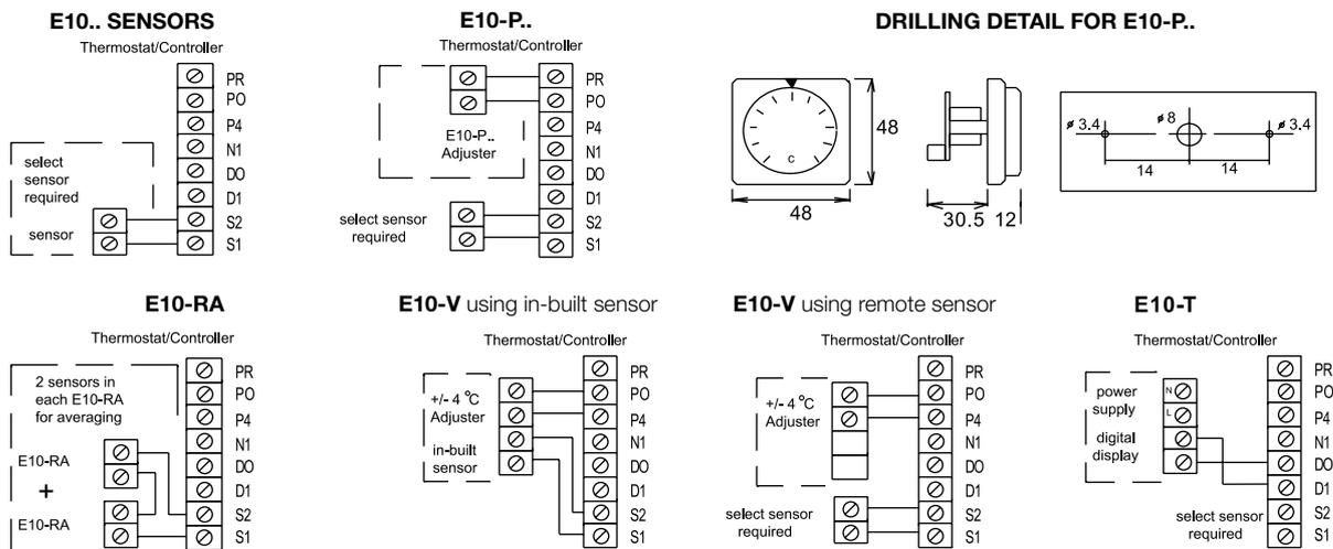
**INSTALLATION:** Terminals 0.5 -2.5mm<sup>2</sup> Max length 100mm. Sensor cable size 7/0.2mm Screened cable is recommended. Keep away from power cables/units which may cause interference. The screen should be earthed at the controller end only.
