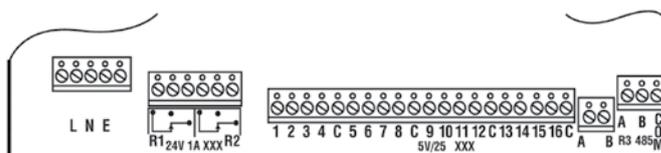
The mains supply should be via a 2pole isolating switch fused at 1A. Use 3x0.75mm sq cable.
